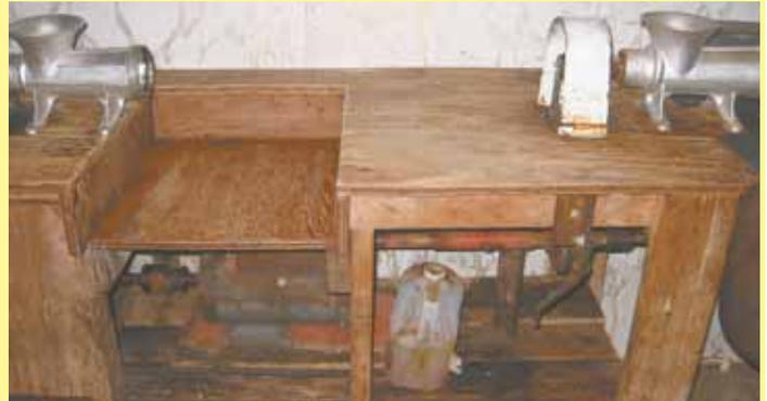
Sickler’s meat grinder is driven by a 220-volt electric motor that powers a driveshaft through the transmission from a Datsun pickup.
