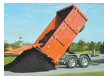
Trailer comes with a remote-controlled jack, double-acting tailgate, and power hoist that lifts up to a 47-degree angle.
