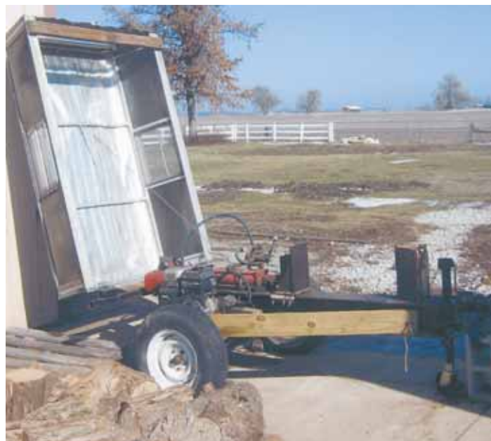
"It looks nice and makes an ideal weather top in any season," says Bill Martin, who used the fiberglass topper off an old pickup as a cover for his trailer-mounted log splitter.
