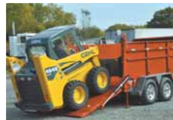
Hydraulic cylinders lift tailgate from the bottom for dumping or lower it from the top, forming a drive-on ramp.
