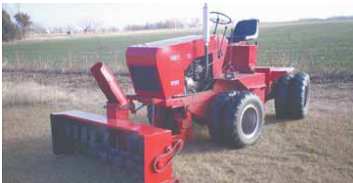
Harold Tribitt wanted a larger snowblower so he used the frame, fan and gearbox from a snowblower he had built earlier as the foundation for a new machine.
