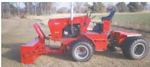
Harold Tribitt wanted a larger snowblower so he used the frame, fan and gearbox from a snowblower he had built earlier as the foundation for a new machine.
