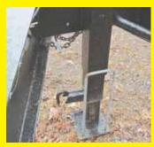
I was tired of reaching for the handle at the base of my trailer jack so I installed an extended handle to the base. I have a spring-loaded lock pin that I can pull out and turn it on the side, raise the base, and hit it with my foot to lock it in the up position. (Larry Goodman, 3200 Welch Rd., Ionia, Mich. 48846 ph 616-755-1473)
