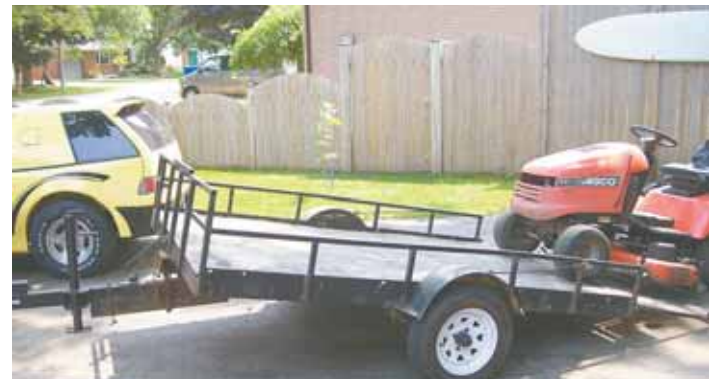
Bruce Riehl converted an old tilting snowmobile trailer into a lawn mower trailer that's easy to load without the mower deck binding up.
