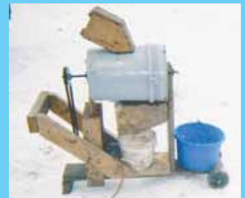
Automatic corn sheller uses an electric motor to belt-drive beater inside bucket.
