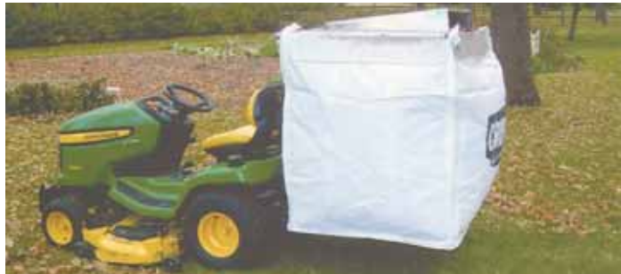
Cal Miner made a high capacity bagger out of a large nylon bulk seed bag that's 4 ft. wide. Bag is supported by a platform made from plywood covered by aluminum.
