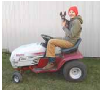
Cameron Messinger went to Northern Tool and bought 10-in. low-speed wheels to mount on front of his garden tractor.
