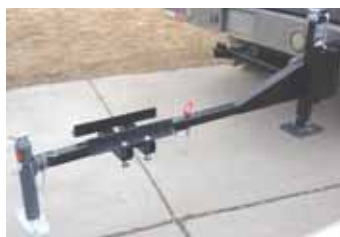
Foldable anvil hitch (shown here without anvil) fits pickup's receiver hitch. Anvil is secured between angle iron brackets bolted to 2-in. sq. tubing. A pair of jacks add stability.
