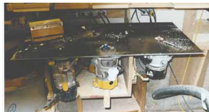
Norm Dufresne put together this portable router table with 4 routers, which are set up with different bits at the right depth for the most common cuts he makes.
