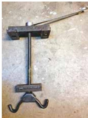
Nathan Fleischer made a piston sleeve puller using the threaded bolt and jaw from a coil spring compressor.
