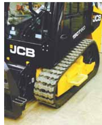
Made from expanded metal and angle iron, access step mounts to side of undercarriage on Houston's JCB tracked skid loader.
