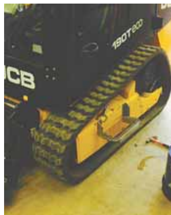
Made from expanded metal and angle iron, access step mounts to side of undercarriage on Houston's JCB tracked skid loader.
