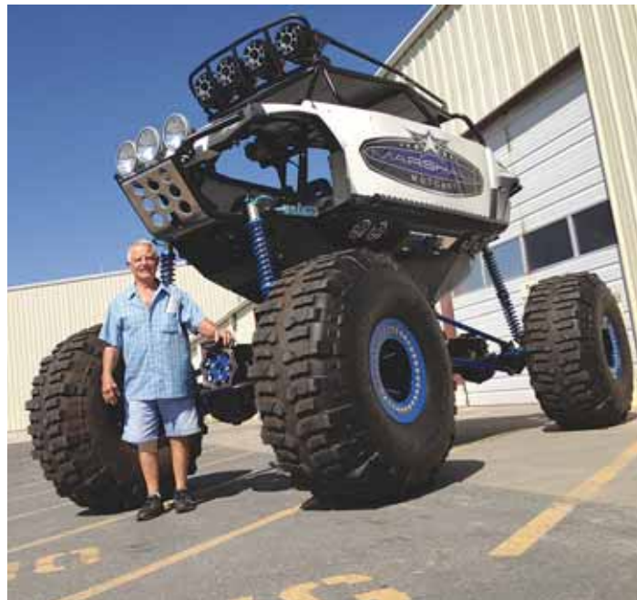
Chris Burke converted a 4-seater Polaris Ranger into this 11-ft. tall "Monster Ranger". It rides on big 54-in. off-road tires and can seat up to 6 people.
