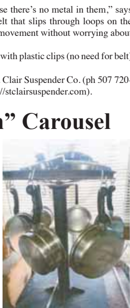
Pots and pans rotate on carousel made from an old bicycle wheel.
