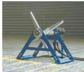
Robert Stahl invented the Sump Saver to solve problems with plugged augers in big bins. Four rotating fingers break up clumps.
