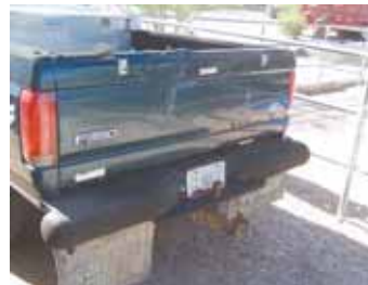
Lloyd McConnell needed a handy supply of emergency air, so he replaced the front and rear bumpers on his pickup with air tanks fabricated from schedule 80 pipe.
