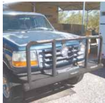
Lloyd McConnell needed a handy supply of emergency air, so he replaced the front and rear bumpers on his pickup with air tanks fabricated from schedule 80 pipe.
