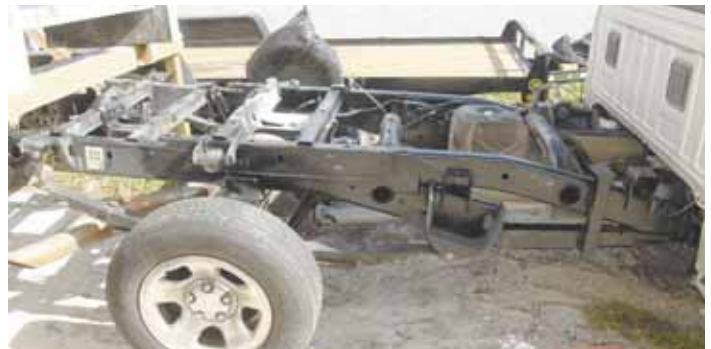
He found a Dodge Ram 2500 and bought just the rear half of the frame and also the rear springs, then welded a new frame together to match the end of the original frame.
