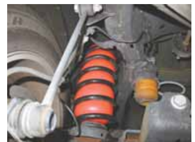
Air Lift 1000 air springs provide up to 1,000 lbs. of load-leveling capacity. They're easy to install and popular with 1/2-ton pickups and SUV's, says the company.
