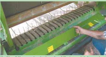
"Leaf Saver" fills a gap to keep hay leaves from falling between baler's rear axle and pickup head.
