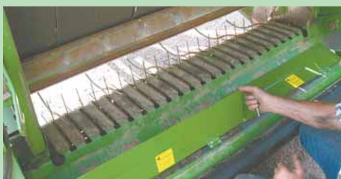
"Leaf Saver" fills a gap to keep hay leaves from falling between baler's rear axle and pickup head.
