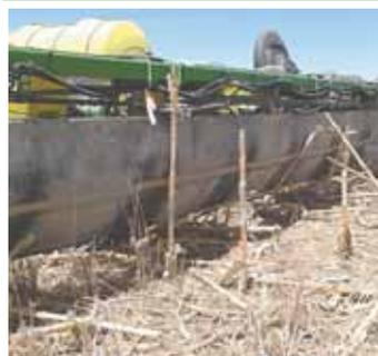
Scott Ravenkamp uses old conveyor belting to protect his planter from stalk damage (left). He also uses 55-gal. plastic drums to make auger hoppers.
