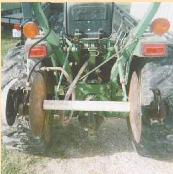
Barbed wire roller mounts on brackets that attach to 3-pt.'s lower lift arms. A PVC pipe and 2 disk blades are used to hold the wire.
