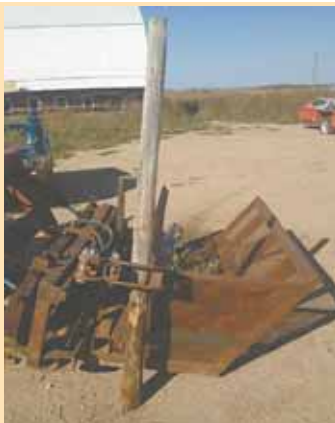
Operator clamps jaw onto post and then raises it straight up with loader. Once post is out of ground, a separate cylinder then rotates post and drops it into metal basket.
