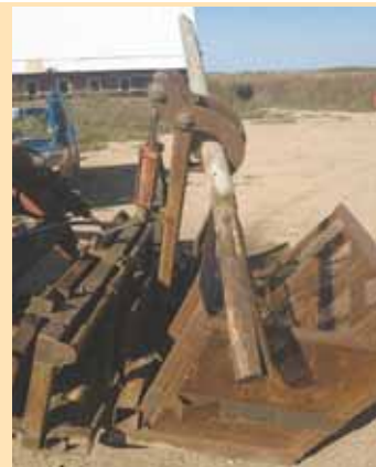
Operator clamps jaw onto post and then raises it straight up with loader. Once post is out of ground, a separate cylinder then rotates post and drops it into metal basket.
