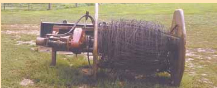
Skid loader-mounted wire winder is designed to roll up posts with the wire. "It'll eat the whole fence up," says inventor Kelly Faeth.
