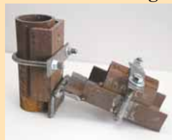
Photo shows one of Hackman's fence brackets U-bolted to short lengths of pipe for demonstration purposes.
