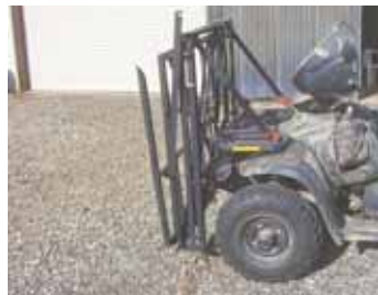
Mathis used 1-in. angle iron to build the attachment, adding hinges to tilt the forks forward to empty the load. When not in use the forks fold up for easy storage.
