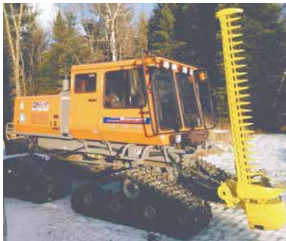
Norman Bennett modified a 7-ft. belly-mounted cutterbar to fit the front of a track-type Sno-Cat. "It's an easy way to mow brush along snowmobile trails," he says.
