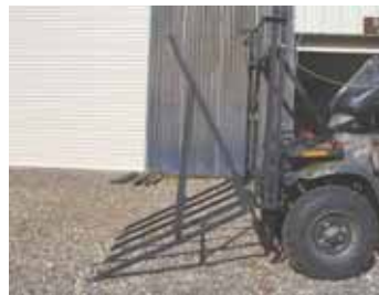
Mathis used 1-in. angle iron to build the attachment, adding hinges to tilt the forks forward to empty the load. When not in use the forks fold up for easy storage.
