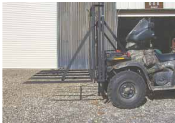
Rondle Mathis says his ATV-mounted brush hauler is small enough to maneuver in wooded areas. It uses the ATV's electric winch and lifts up to 18 in. off the ground.
