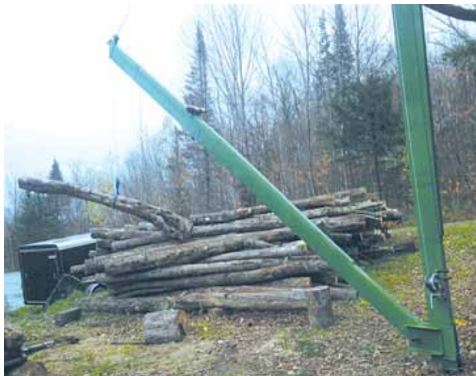
Home-built 30-ft. tall crane is fitted with a 28-ft. gib that's free to swivel on an underground base and is fitted with a 5,000-lb. electric winch. Bennett uses a remote control to lift log off pile, then manually rotates the gib and lowers the log onto a conveyor for splitting.
