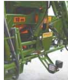
Blue LED sprayer boom lights make it easy to visually check nozzles and spray patterns from the cab at night.
