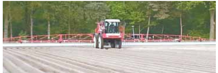
Wingsprayer works with very fine droplets that are protected by a windshield. It results in reduced chemical use and less spray drift.
