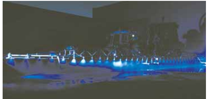
Blue LED sprayer boom lights make it easy to visually check nozzles and spray patterns from the cab at night.
