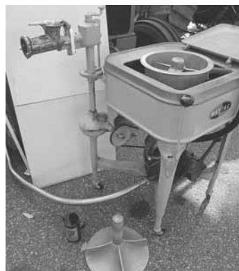
Rare washing machine could also be used as a butter churn ice cream maker - or, you could fit a standard meat grinder onto the wringer post.
