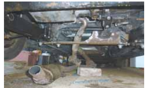
He extended the motor mount to accommodate the narrower engine and transmission, and added a wishbone brace that bolts onto the transmission.
