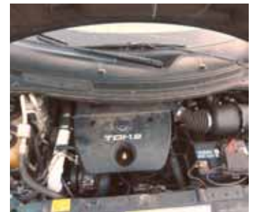
Matt Eby repowered a Ford Windstar van with a VW diesel engine, boosting mileage to as high as 42 mpg.
