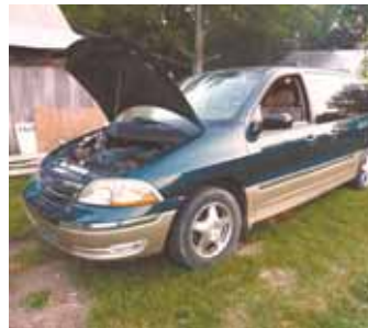
Matt Eby repowered a Ford Windstar van with a VW diesel engine, boosting mileage to as high as 42 mpg.
