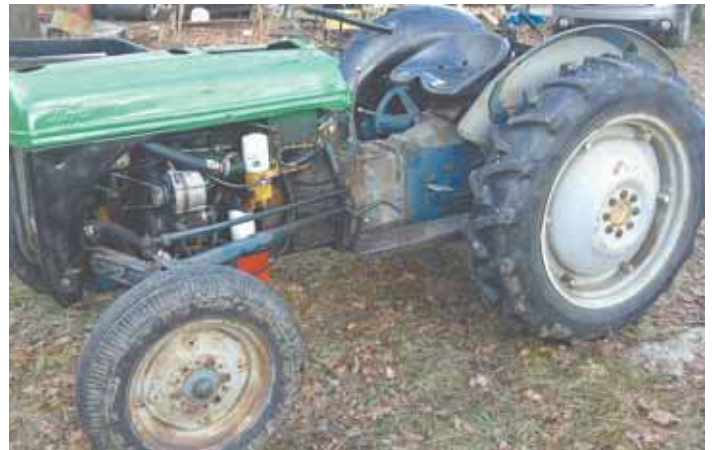
Al Rutkoski repowered a Ferguson TE20 tractor with a 1.6-liter VW diesel engine from a VW Rabbit. "It's fuel-efficient and puts out about 48 hp at 4,000 rpm's," he says.
