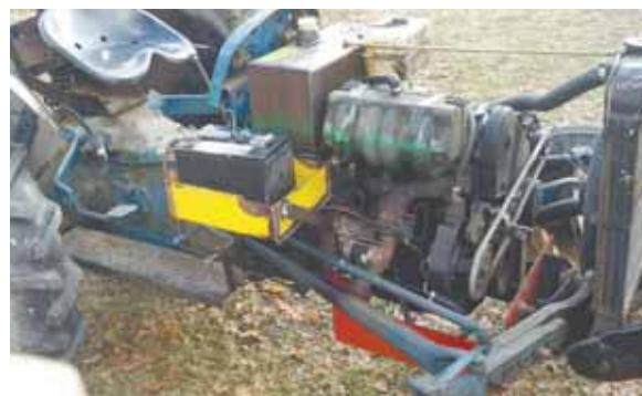
Al Rutkoski repowered a Ferguson TE20 tractor with a 1.6-liter VW diesel engine from a VW Rabbit. "It's fuel-efficient and puts out about 48 hp at 4,000 rpm's," he says.
