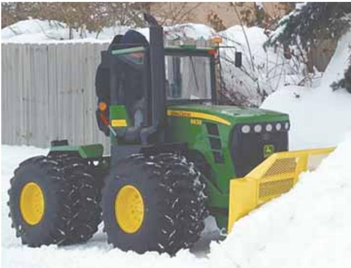
Don Campbell started out with the frame, axles and engine from an old Steiner front-mount riding mower to build this half-scale articulating Deere 9630 4-WD tractor.
