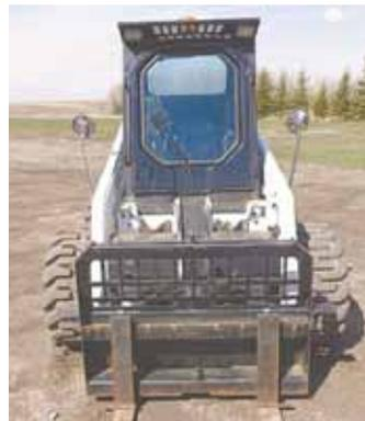
The 6-in. dia. mirrors have a convex shape and are designed to mount on both sides of the operator.
