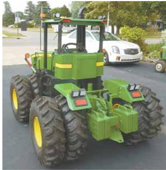
He lengthened the mower's front and rear frames and made new fenders, fuel tank, and hood. "The cab is proportional to the tractor. It looks factory-built," says Campbell.
