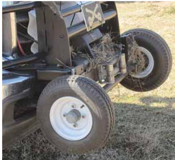
Anderson made a bale unroller by mounting the wheels and axle off an old trailer on front of his pickup. The wheels, spaced 4 ft. apart and 30 in. off the ground, spin freely.
