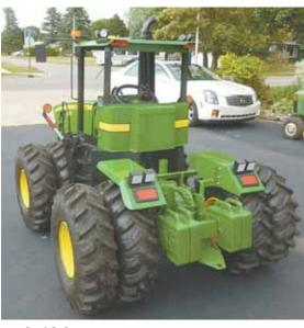
He lengthened the mower's front and rear frames and made new fenders, fuel tank, and hood. "The cab is proportional to the tractor. It looks factorybuilt," says Campbell.
