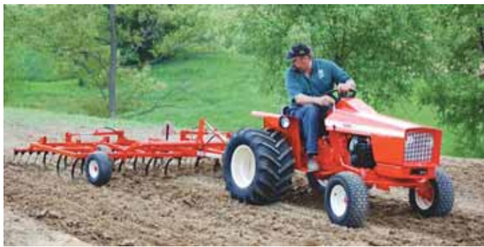
Steve Kauffman built an 11-ft. field cultivator for his restored 1972 Allis Chalmers 616 garden tractor. "It's made to scale and is bigger than anything on the market," he says.
