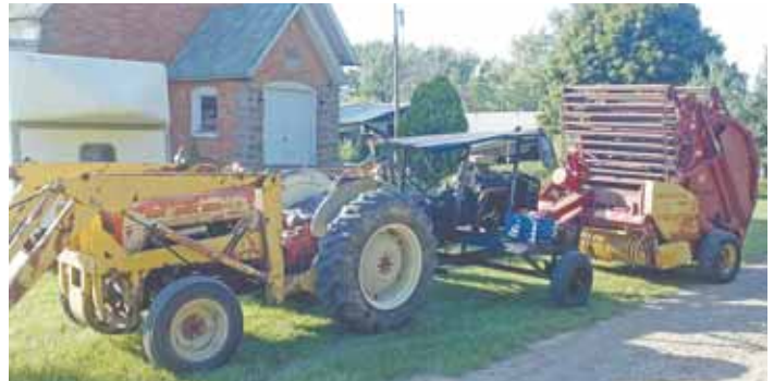
Rutkoski's small Ford tractor didn't have enough power on its own to make full-size round bales. But it's no problem making them with a tow-behind pto cart powered by a Chevy 350 engine.
