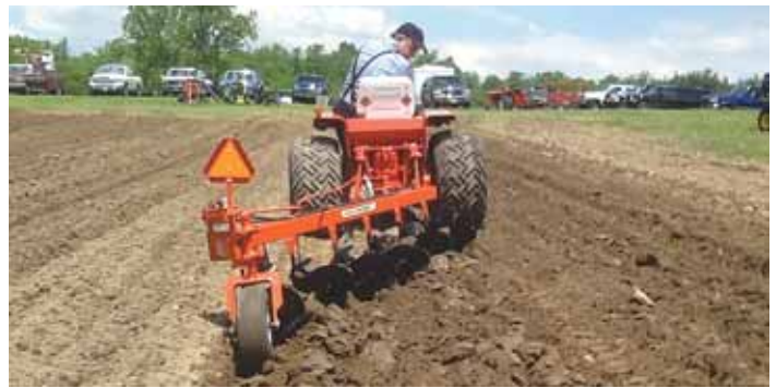
Kauffman's friend Amos built this 3-pt. mounted, 6-bottom moldboard plow for his restored AC 616 tractor. The plow has 8-in. moldboards and covers a 4-ft. wide swath.
