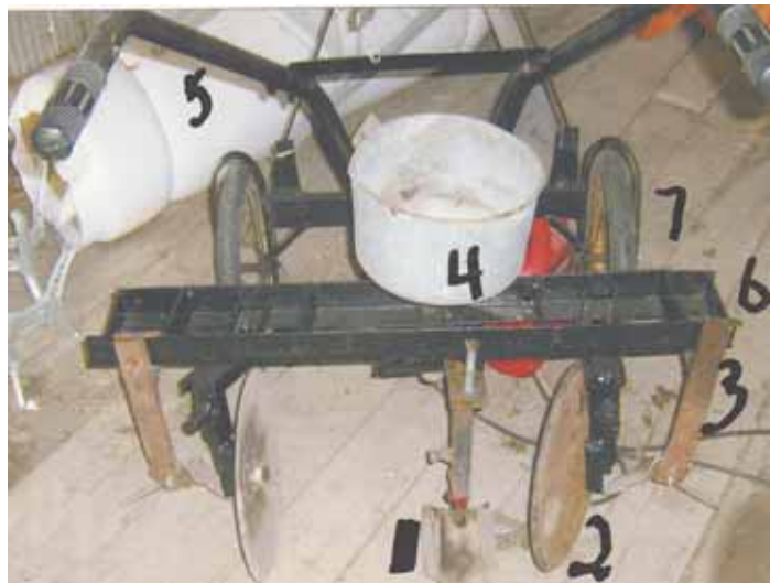
Multi-purpose implement makes growing potatoes an easier job. Components include: 1. Fertilizer spreader plate; 2. Hilling discs; 3. Cultivator shovels; 4. Fertilizer funnel; 5. Handles from a rototiller; 6. Toolbar; and 7. Child-size bike tires.
