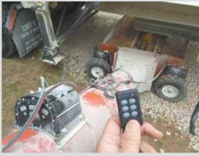
Remotecontrolled Auger-Jogger makes it easy to move swing hopper into place under trucks and wagons.
