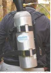
Arctic Frostbite sprayer converts liquid CO, into dry ice frost that kills weeds fast. The CO, cylinder can be used with a backpack harness, if desired.
