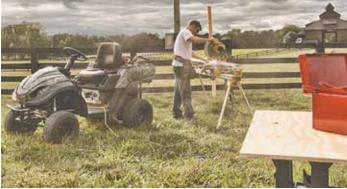
Removing the mower deck transforms the gas-electric Raven into an off-road utility vehicle. Once at a remote site, it can be used to power tools.
