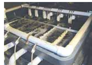
Recirculating system uses 40 hp motors to oxygenate the fish tanks. Air diffusers along bottom of tanks create 2 opposing flows of water.
