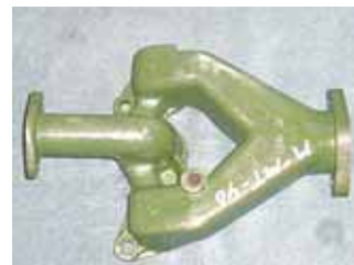
Shepard's Tractor Parts sells new, used and reproduction parts, primarily for pre-1960 2-cyl. tractors. Photo above shows the manifold for a Deere M.
