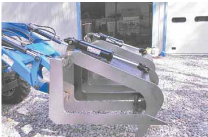
Grapple fork measures 71 1/2 in. wide and has 40-in. long tines at the bottom spaced 8 in. apart. A pair of 10-in. hydraulic cylinders are used to raise and lower the shanks.
