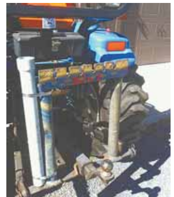
Chain at end of log catches in one of several notches at top of 3-pt. mounted lifter.
