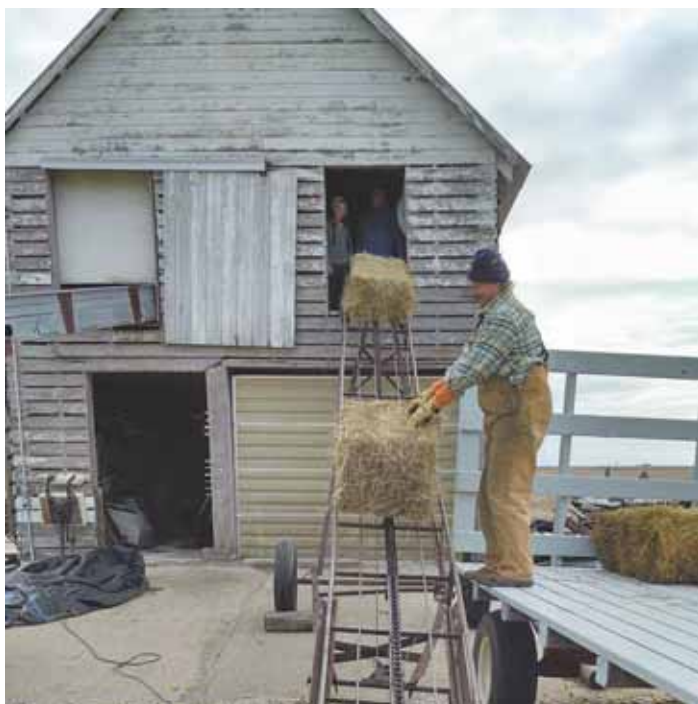
Brett Hundertmark reversed the wires on an 850 rpm electric motor and mounted it on this elevator to run the chain backward. "The bales come down nice and slow, making them easy to stack on the hay rack," he says.
