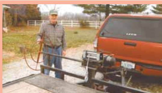
John Eilers fitted the hand-operated winch on his implement trailer with a big drive wheel, making it easier to crank.
