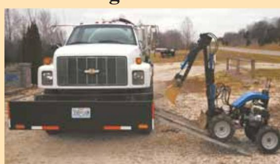
truck. He extended the frame about 3 ft., providing more than enough space for the 32-in. wide backhoe.
