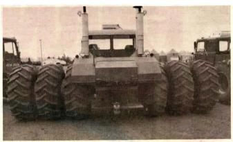
Each of Earl Laufer's three truck-tractors can be fitted with triples that result in a total working width of 21 ft. Laufer, who farms near Hettinger, N. Dak., built his first tractor in 1963. He uses Euclid industrial rear ends together with whatever semi-truck cab and frontend he can find. He's built three for his own use and has helped neighbors build their own, too.
