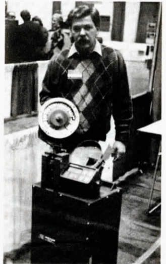
Deere finger pickup unit quickly clamps to test stand for elevation.
