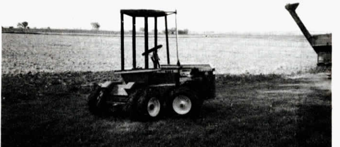
Mini-tractor features front and rear duals, and articulated steering.
