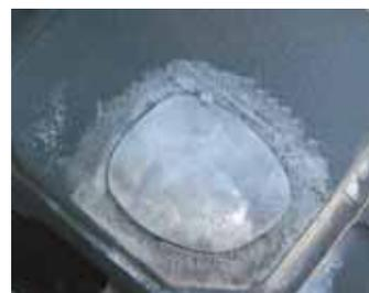
**Lock-N-Stitch can also be used to make patches by drilling a series of holes.**
