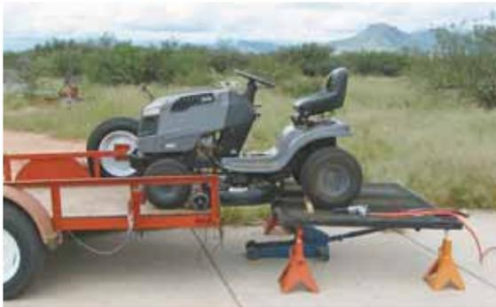
Mower is suspended between trailer and ramp, allowing Niesel to easily change blades on the deck.
