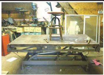
Jim Borden converted an old hospital bed into an adjustable height workbench. He uses a foot pedal to raise and lower the unit anywhere from 16 to 34 in.
