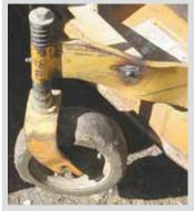
Robert McMahon, Knoxville, Tenn.: "We use a small 4-WD Kubota loader tractor and a 3-pt. mounted, 6-ft. Woods finish mower to cut grass. We farm a lot of rough terrain and when we made a sharp turn with the tractor, we accidentally bent the spindles on the mower's caster wheels.
