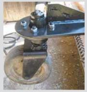
spindles and hubs are much stronger than the factory ones on the mower. The photos show 'before and after' photos of the conversion.
