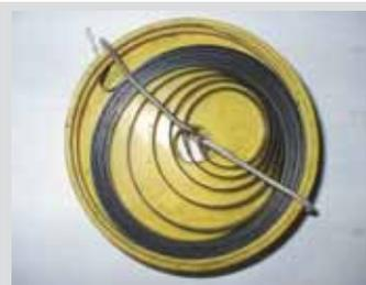
**Dwayne Oxford, Holladay, Tenn.:** "Here's how I store good pull-start springs off small engines. I drill a hole in the center of a suitable size lid, then wind the spring into the lid, beginning with the outer end. Then I thread 14 or 16-ga. solid copper wire through the hole and across the spring to keep it in place. I also label the top of the lid with the name of the motor it came out of."
