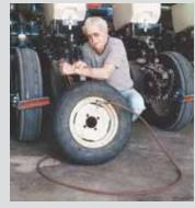
Raymond Werner, Winfield, Iowa: "I use an old tire as an in-field air transfer system. It lets me fill a flat tire in the field with enough air that I can get back to my shop or to a tire repair garage. All I do is attach one clip-on air fitting to the tire's valve stem and another fitting to a short length of hose.
