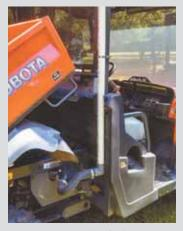
Lloyd R. Lucas, High Springs, Fla.: "I was going through a lot of air filters on my Kubota UTV until I made this change. I ran a long piece of pvc from the filter up through the roof of the vehicle. Pulls in clean air. Big improvement and I'm running with a clean filter much longer.
