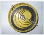
Dwayne Oxford, Holladay, Tenn: "Here's how I store good pull-start springs off small engines. I drill a hole in the center of a suitable size lid, then wind the spring into the lid, beginning with the outer end. Then I thread 14 or 16-ga. solid copper wire through the hole and across the spring to keep it in place. I also label the top of the lid with the name of the motor it came out of."
