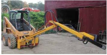
Chainsaw at end of 2-section boom is chain-driven by a motor that operates off the remote outlets on Mickley's skid loader.
