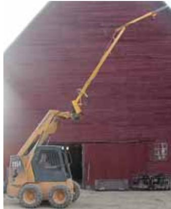
Skid loader-mounted saw has a maximum reach of about 22 ft.
