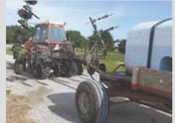
Liquid is supplied to machine's toolbar from a 1,600-gal. tank mounted on an all-steer wagon.
