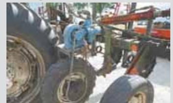
John Blue ground-driven pump is mounted at front of toolbar.
