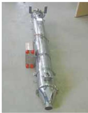
Heat Collar channels exhaust through a pipe filled with small tubes, capturing otherwise wasted heat from stationary engine exhausts.
