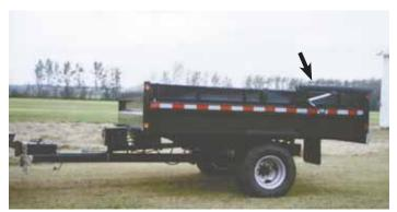
Dump trailer's tailgate is operated by 2 small hydraulic lift cylinders. As they're extended, they slide the entire tailgate assembly up above the trailer.
