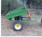
Irvin Wehman, Jr., built this dump trailer using the box off an old Deere Gator utility vehicle. An 8,000-lb. hydraulic cylinder is used to raise and lower the box.
