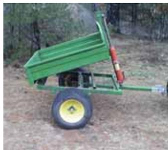
Irvin Wehman, Jr. built this dump trailer using the box off an old Deere Gator utility vehicle. An 8,000-lb. hydraulic cylinder is used to raise and lower the box.
