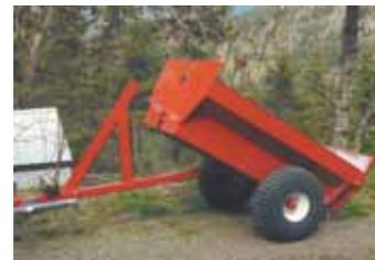
An electric winch mounted on the tongue is used to dump the trailer.
