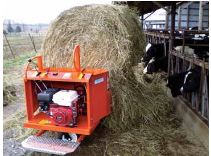
Self-propelled Bale Unroller unrolls hay to the left or right. The operator stands on a platform at the rear of the cart and uses joystick controls.
