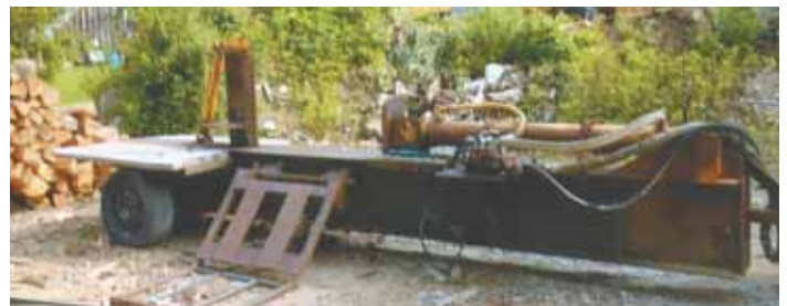
George Young, Jr., and his friend Joseph Morin built this massive wood splitter that's powered by a 300 hp Mack semi truck.
