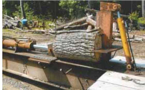
George Young, Jr., and his friend Joseph Morin built this massive wood splitter that's powered by a 300 hp Mack semi truck.
