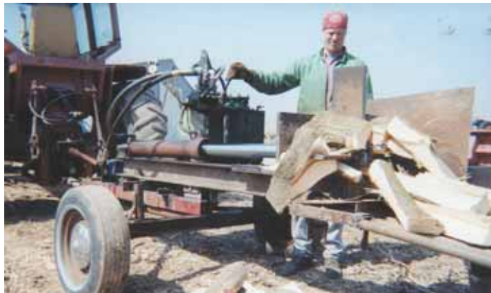
Norman Zemlicka used the hydraulic pump from a garbage truck to build this wood splitter.
