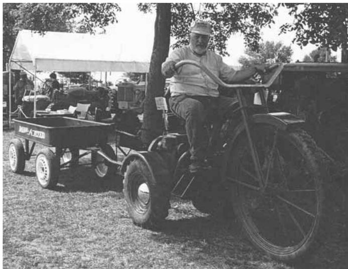
Wayne Timm sometimes drives his "big wheel" tricycle at antique tractor shows. The tricycle's 44-in. spoked front wheel is off an old Case ground-driven hay rake.
