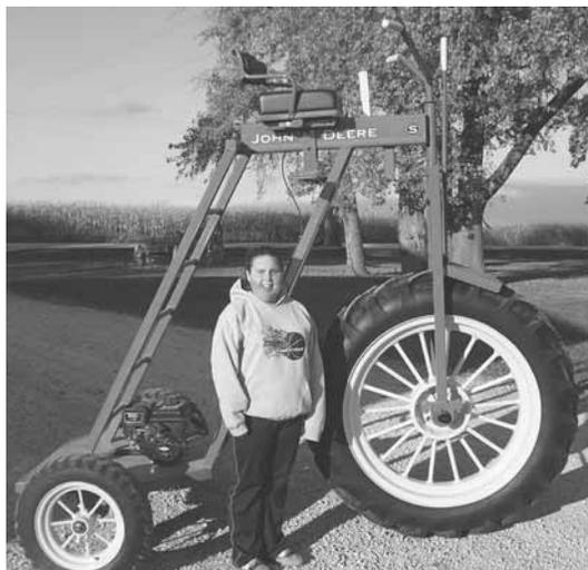
Sarah Rasmussen and her dad built this 10-ft. tall trike complete with a 36-in. high front wheel. It's powered by a 5 1/2 hp Briggs & Stratton engine.
