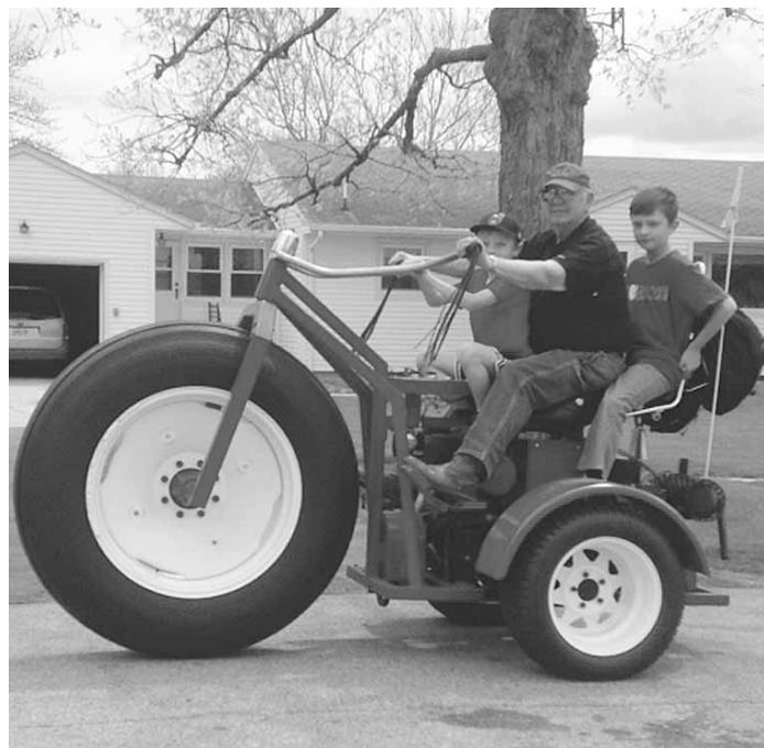
Arvid Miller's giant 3-wheeler sports a big front wheel with an 11.75 by 28-in. tire. The rear wheels are driven by a Kohler 25 hp, 2-cyl. engine.
