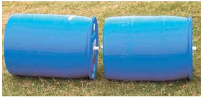
Barrels are strung together by lengths of pvc pipe and sealed with silicone to stay watertight.
