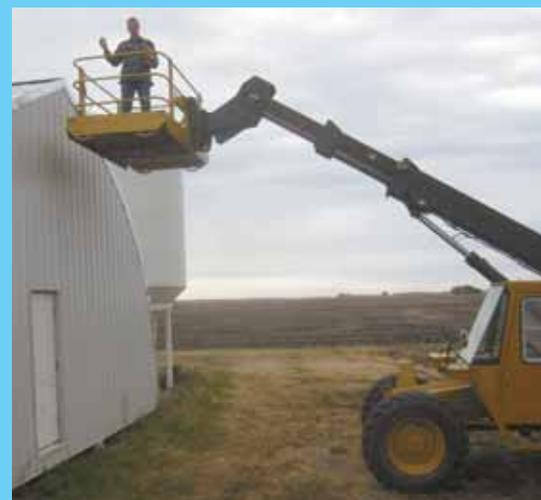
Using an inexpensive wireless remote control, Leroy Groening can start, stop, raise, lower, extend and retract the boom on his Cat Telehandler.
