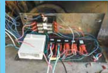
Groening bought the 12-button remote handset transmitter and receiver on eBay (on left) and built a control board with relays (on right that manages telehandler function switches.
