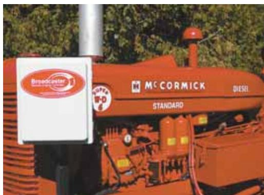
Remote controller can start a tractor's engine, activate the pto and control rpm's.
