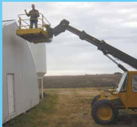
Using an inexpensive wireless remote control, Leroy Groening can start, stop, raise, lower, extend and retract the boom on his Cat Telehandler.
