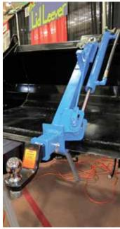
Operated by a hydraulic cylinder, bucketmounted hitch swings down 90 degrees and locks onto bucket's cutting edge.
