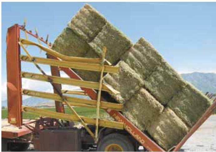
Garry Brown modified his self-propelled small bale stacker wagon to haul and stack up to 10 big square bales at a time.
