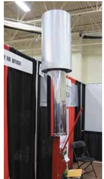
Chimney "diffuser" knocks down the wind velocity at top of chimney by introducing outside air at top of flue.
