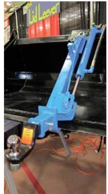
Operated by a hydraulic cylinder, bucket-mounted hitch swings down 90 degrees and locks onto bucket's cutting edge.
