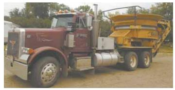
They repowered the semi tractor with the 410 hp Cummins diesel that originally powered the grinder, so now the engine supplies power for both the truck and the grinder.
