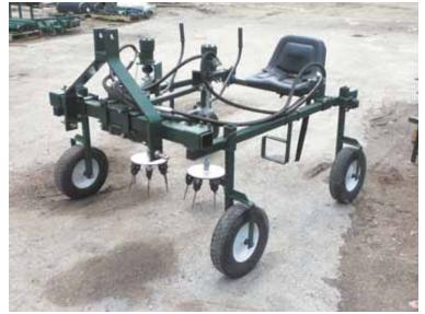
Willsie Equipment's 3-pt. mounted Hydraweeder allows a person to sit and operate rotating digging heads around plants.
