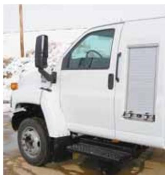
Roll-up door behind driver's door on extended cab pickup makes for easy access to storage space.
