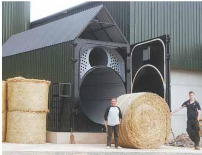
Boiler uses big 7-ft. dia. bales made by a Krone high density baler and holds 3 bales at once. The heat they produce is equivalent to burning 370 gal. of diesel fuel.
