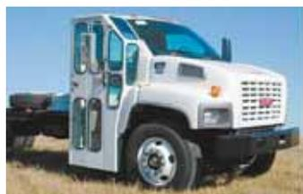
Cab re-do's can include dual steering with stand-up or seated right hand steering and controls.
