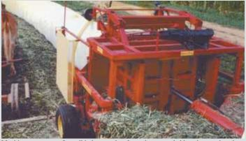
Machine compresses 8 small bales together from the top and sides, then pushes them through a 4-ft. sq. chamber which leads to the wrapper.
