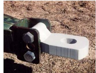
"Rigid replacement tongue" comes with an elongated 2 1/4-in. long hole and an extra bolt that keeps the unit in a rigid horizontal position. Photo at right shows original floppy tongue hitch design.
