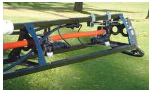
GPS-guided spraying system turns spray nozzles on or off individually to virtually eliminate over and under spraying.
